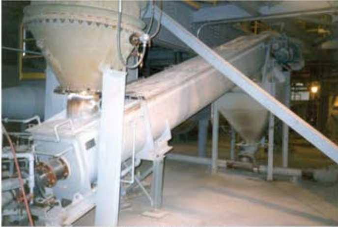
"HOLO-SCRU" Ash Cooler handling 2000 lb/hr of bed ash and sand material
