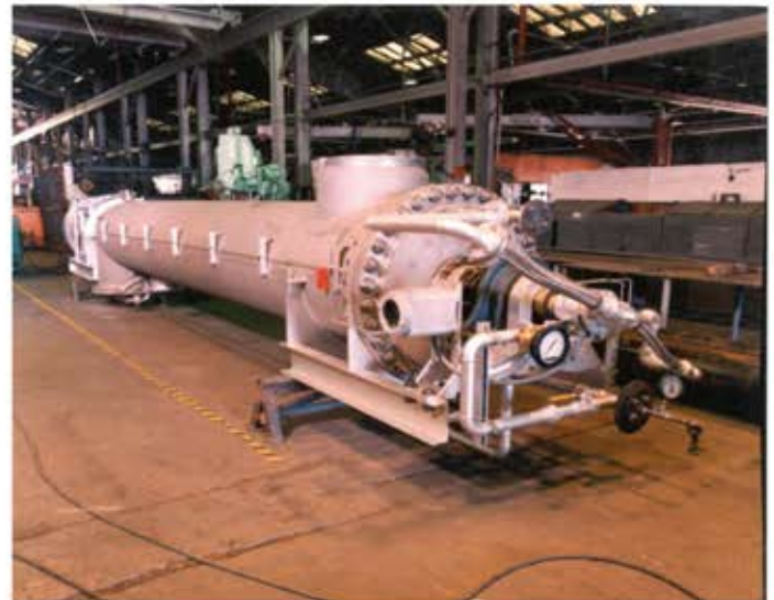
Special Application of "HOLO-SCRU" Ash Coolers used in Pressurized CFB handling 3,000 lb/hr of bottom ash and sand at 250 psig internal pressure
